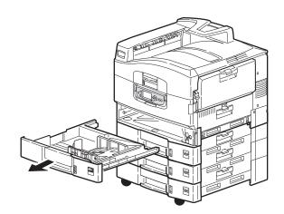
**4.** Gaining access through the gap left by Tray 1, wipe the 3 paper feed rollers (2) with a soft cloth lightly moistened with water.
