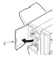
**3.** Continue to turn the lower knob (3) clockwise until any jammed paper is completely ejected.
