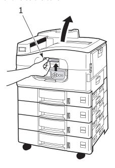
To close the top cover, push gently (1) until the cover stops midway and then push harder (2) to close the cover completely. Ensure that the cover is securely closed.
