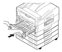
**10.** If you detached a Finisher unit to gain access to the duplex unit, replace the Finisher unit.
