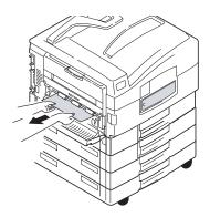
**4.** Operate the levers (3) and pull out the duplex unit.
